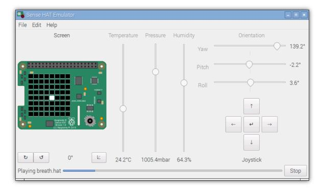
During playback, the sensor sliders will move according to the data in the recording but will be disabled (to prevent the user affecting the replay). At the end of the replay (or immediately after termination of playback), the sliders will be left at their present positions and re-enabled.
