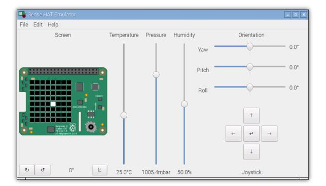
The main window is divided into four parts. At the top left is a visual representation of the Sense HAT. Scripts using the emulator library (*sense\_emu*) to set the HAT's LEDs will display the result here. Immediately below the LEDs are the rotation buttons which rotate the view of the HAT. These buttons also affect the action of the joystick buttons (covered below).
